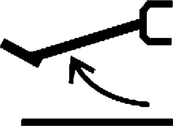
The symbol shows a crane stabilizer arm tilted upwards. A curved arrow points from the base towards the top of the arm, indicating the direction of movement. A thick horizontal line below the base represents the ground.      | Стабилизатор - подъем         |
